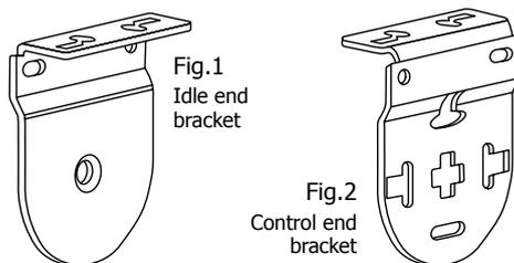
**1.** To work out the distance required between each bracket you will need to first measure the fabric width, e.g. 1500mm. Add to this an allowance for the control and idle end of 33mm, e.g. = 1535mm.
