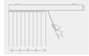
Twist the wand to tilt the slats in either direction to
