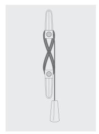
Breakaway cord condenser is pre-fitted to the lift cords so that when a horizontal force is applied to the cords entering the condenser it safely breaks away eliminating any hazardous loops.
